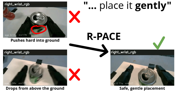
Fig. 1: Teaser. A frozen zero-shot VLA can complete the task while still violating a soft execution preference such as place it gently . Left and middle: representative base-policy failures with rough final placement. Right: R-PACE cuts the risky tail of the chunk, refreshes, and improves execution quality.
